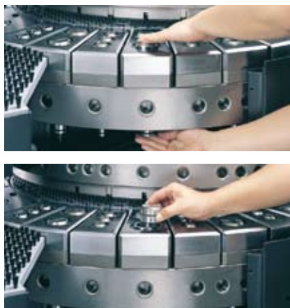
Faster, easier tool changing in the Z turret with the help of ejector pipes
